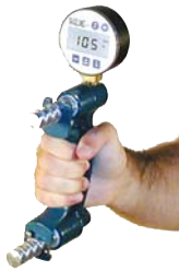
060094 Gives accurate grip strength readings without the subject being able to "feel" the handle move.
